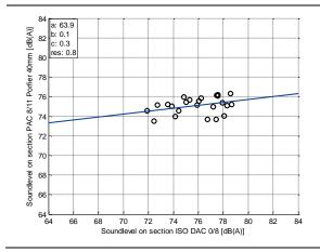
Relation between rolling noise levels of a series of tyres on ISO 10844 surface relative to the rolling noise of the same tyres on a porous asphalt concrete surface. Slope =0,1, correlation=0,3 (Ref [6])
