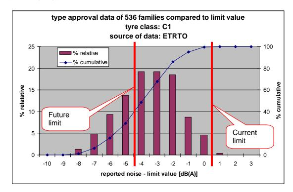
figure 11 Statistical distribution of type approval results of tyres compared to the current limit (EC2001/43). By the end of 2012 the limit will be reduced by 4 to 5 dB (EC661/2009). An estimated 40% of the current tyres fulfil these limits. The other 60% will have to be improved.
