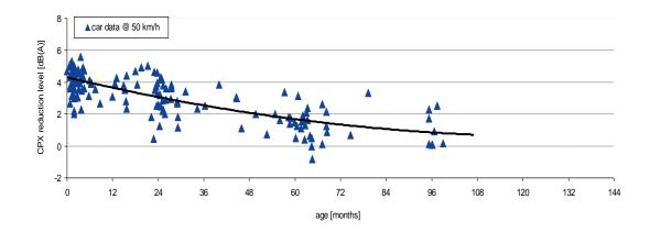
figure 16 Measured data of noise reduction of thin layer surfaces as a function of age (ref. [16]).
