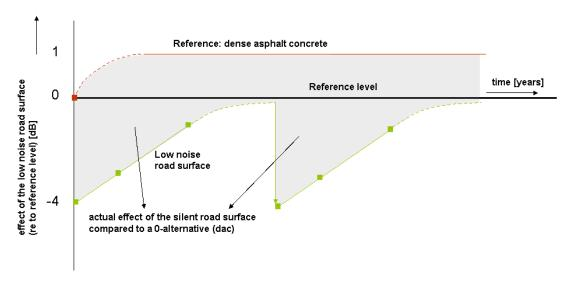
figure 17 Time line of the noise reducing effect of low noise surface compared to a standard surface. The averaged overall effect in this example is still 2,9 dB, even when the final reduction value is close to zero.
