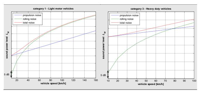
figure 4 Level of rolling noise and propulsion noise as a function of speed. The red curve presents the total sound level. Left: light vehicles, right: heavy vehicles (≥3 axles). Ref.[1]
