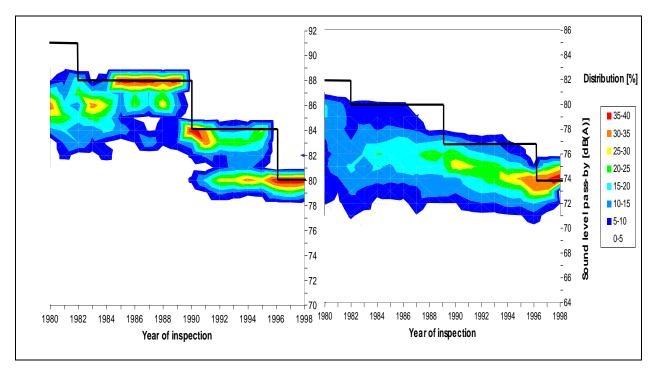
figure 7 Results of vehicle type approval test results during fur stages of tightening of limit values. Left: trucks, right: cars.
