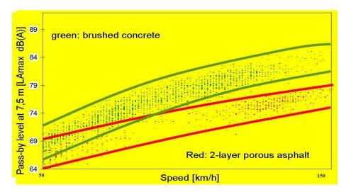
figure 14 Pass by levels (La max at 7,5 m distance) of passenger cars on a 2-layer porous road surface and a fine brushed concrete road surface. The drawn lines indicate the level of the quietest and the noisiest passages.
