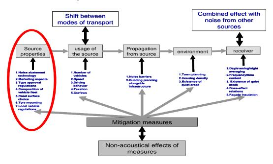
figure 3 Scheme of the process leading to sound exposure and annoyance of the population. Indicated are the measures operating on the several steps. The red circle indicates the focus of this report.
