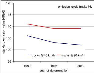
figure 8 Development of emission values of Dutch vehicle fleet. Data from 1980, 1995 and 2010 measurement campaigns.
